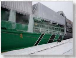
the hatches can't be opened and the containers are frozen solid. even frozen vehicle weighbridges are constantly being put out of commission by ice and frost.
